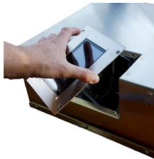
Remove 4 Screws and Reverse the Control Panel 180 Degrees to Down- right (For Wall Mount Installations) Position*
